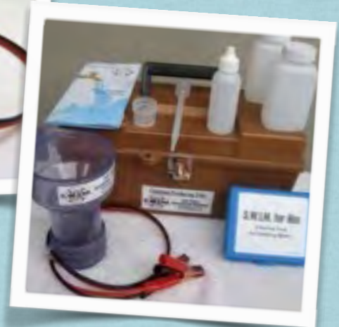
A CPU, mixing bottles, and a test kit fit nicely into a carrying case for ease of use.
